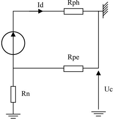
$$I_d = \frac{0,8 \times V \times S_{ph}}{R_{ph} + R_{pe}} = \frac{0,8 \times 230}{2 \times 0,36} = 255 \text{ A}$$
